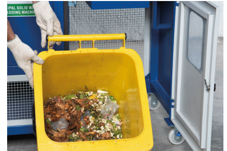
Switch off Motor & take out shredded waste collected in bin
